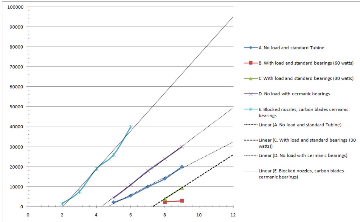
The graph above shows the turbine in a number of configurations. As standard the turbine can spin at the speeds indicated on line A (5 to 9 CFM) and with a bulbs connected 8 to 9 CFM is required to power them, this is shown on line B. Changing the bulbs from 60 watts to 30 watts results in the requirements shown in line C.
